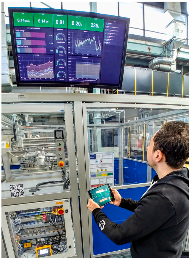
Fig. 7. The legacy loop station level dashboard (on both hand-held device and display screen).
