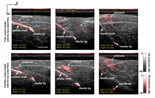
**Figure 6.** Overlaid Photoacoustic (PA) and Ultrasound (US) images acquired during in-plane needle insertions into a pork joint tissue ex vivo with a fully coated needle and a partially coated needle (tip-coated fibres inside the lumens). Blue arrows denote arc-shaped artefacts from the needle tip. Images were obtained from real-time reconstructions and displayed on a logarithmic scale. All the images have the same scale bar of 1 cm.
