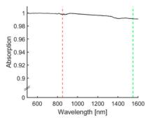
**Figure 3.** Absorption spectrum of CSNP-PDMS nanocomposite deposited onto the distal end of an optical fibre with absorption highlighted at 850 nm (dashed red line) used for PA generation of needle exterior and 1550 nm (dashed green line) used for optical ultrasound generation of the fibre tip.
