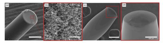
**Figure 2.** Scanning electron microscopy (SEM) images of the coating on the end face of the optical fibre where (**a**) is the CSNP coating, (**b**) is a magnified view of the CSNP nanostructure, (**c**) is the CSNP-PDMS bilayer nanocomposite coating, and (**d**) is a magnified view of the CSNP-PDMS coating. Scale bars are 200  $\mu$ m for (**a**,**c**), 5  $\mu$ m for (**b**), and 100  $\mu$ m for (**d**).
