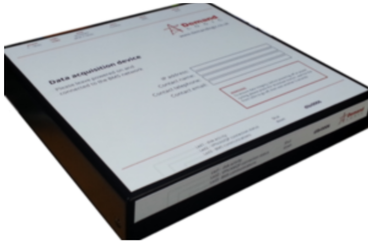
FIGURE 3.2: Data acquisition device (DAD): a company made device for building's data collection.
