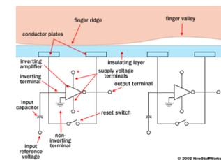
C) Capacitive fingerprint sensor measurement principle [8]
