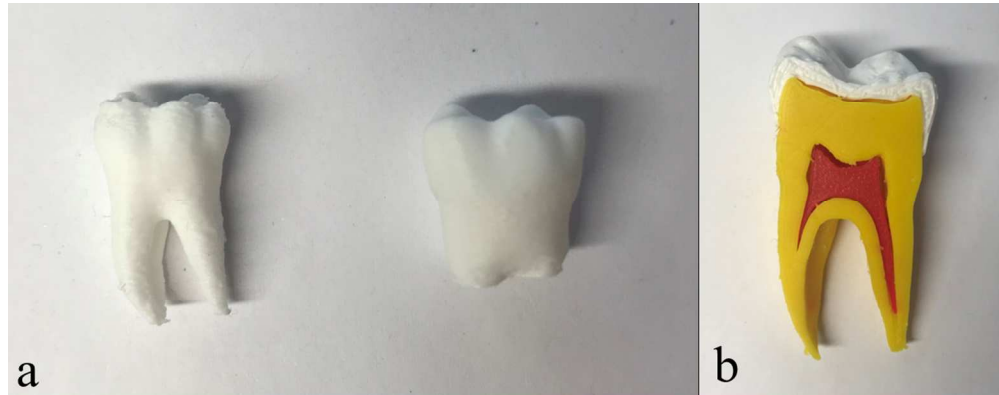
Fig. 4. 3D printed mandibular first molar (a) both natural and artificial molar in PLA, (b) natural molar in multiple materials, PLA for enamel, TPE for dentine and pulp cavity.
