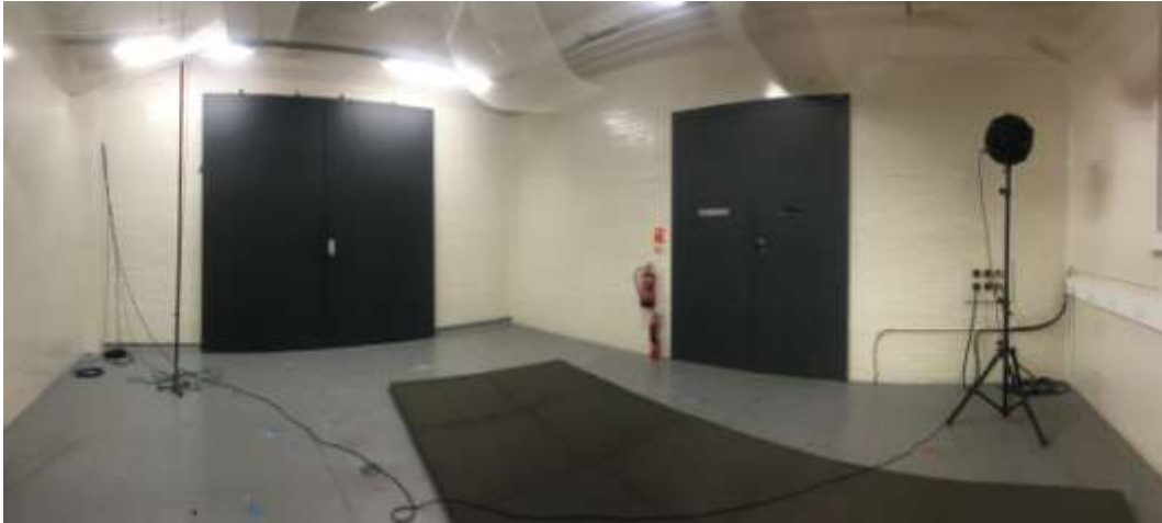
Figure 3. Alternative transducer heights in the LSBU Reverberation Chamber with sample
