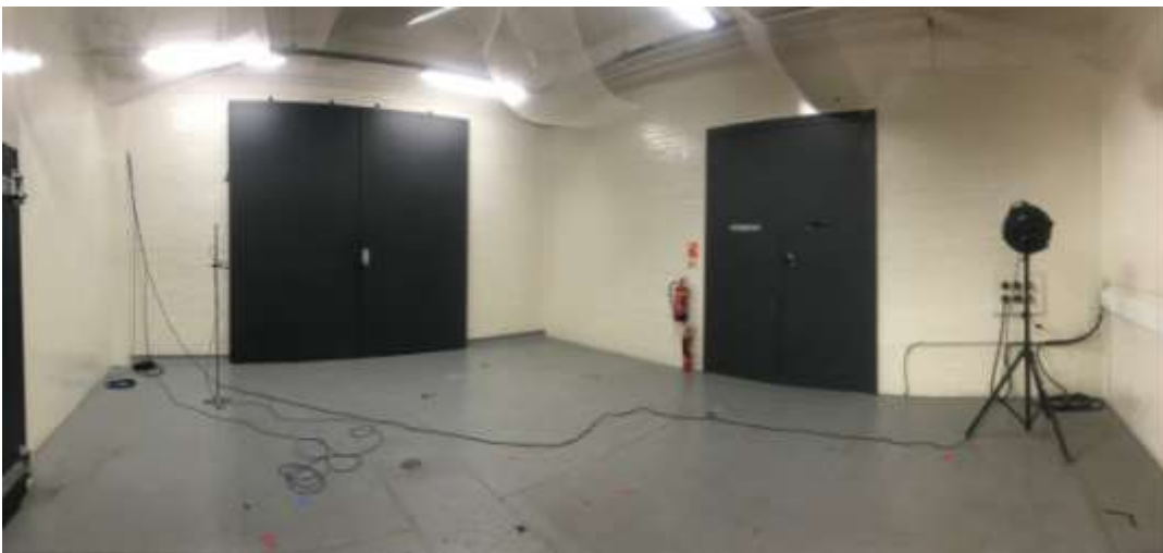
Figure 1. ISO 354 standard transducer heights in the empty LSBU Reverberation Chamber
