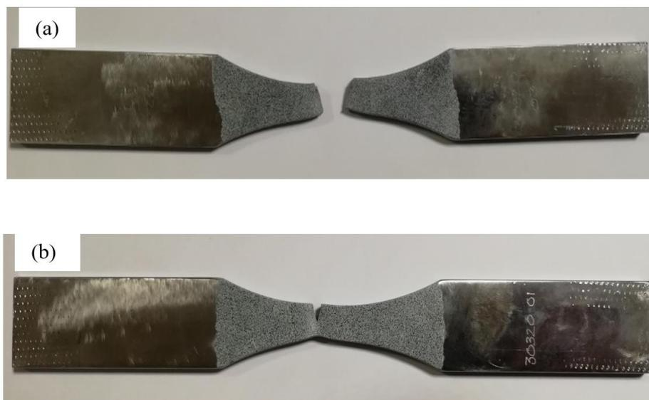
Figure 4-22: (a) Third specimen at the end of test (b) Fourth specimen at the end of test.
