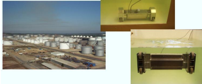
Figure - 6 'Swimming' robot for tank inspection which can automatically change surfaces, scanning the entire floor area and then climbing the tank walls
