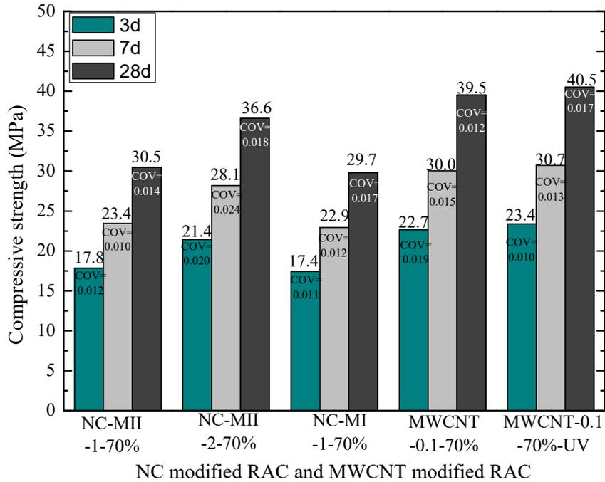
Fig. 15 Compressive strength NC modified RAC and MWCNT modified RAC
