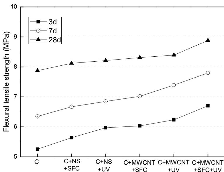
Fig.8 Flexural tensile strength of cement mortar
