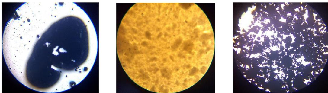
310 (a) MWCNT liquid (b) MWCNT liquid with surfactant (c) MWCNT liquid with UV
