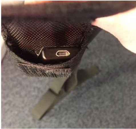
Figure 3.4: accelerometer taped in the pouch
