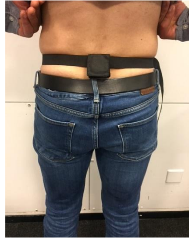
Figure 3.3: the belt worn around the waist at the L4-L5 spinal level
