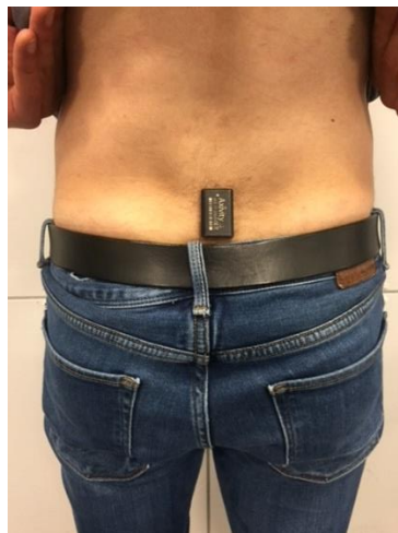
Figure 3.2: Tape method of mounting the accelerometer to the spinal level L4-L5 using double-sided hypoallergenic sticky tape
