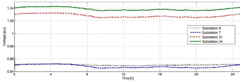
**Fig.3.** Voltage profile for substations 7-9-22-24
