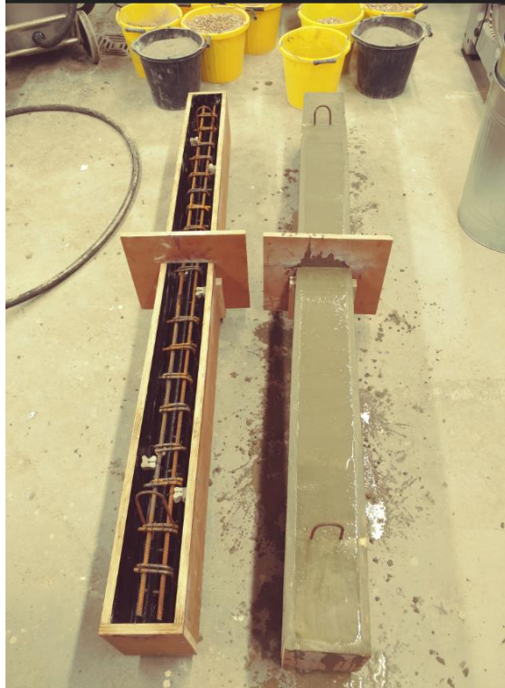
Fig. 3: Beam concrete casting
