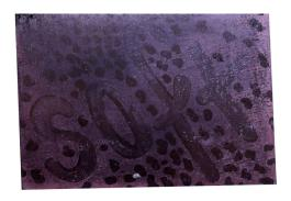
Figure 4: The word "SOFT" is lightly etched into a copper board.
