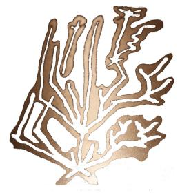
Figure 5: A cascading structure has been etched from a copper board and additionally been cut out in Photoshop so that just the tree shape appears as if surrounded by copper.
