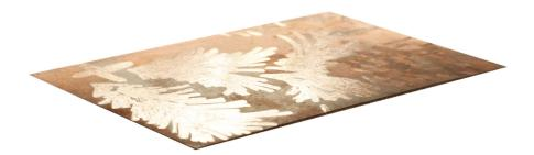
Figure 6: On a copper board photographed from an angle, multiple treelike structures, the non binary trees, have been etched away. They are more shiny than the rest of the copper.
