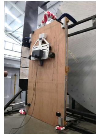
**Figure 17.** Climbing robot tested on vertical wall.
