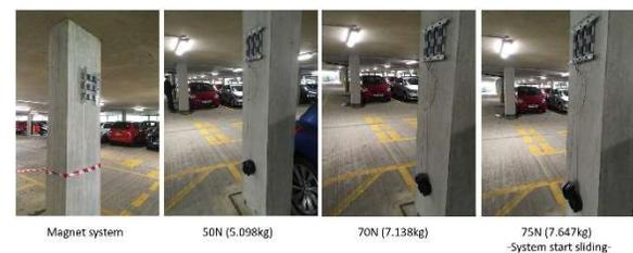
**Figure 11.** Test on a real reinforce concrete structure: car park column.
