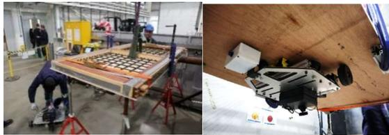
**Figure 16.** (Left) The wall placed horizontally, (Right) Climbing robot on the wall showing that the adhesion force is sufficient to support the payload.
