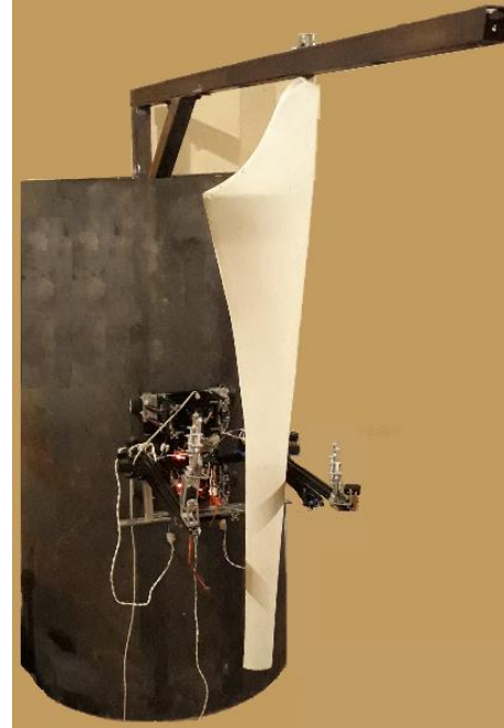
Figure 4.28 Wind turbine tower and blade with the climbing robot
