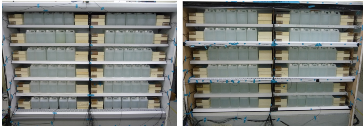
Figure 2: Photograph of cabinets loading during the test; conventional cabinet on (left) and short air curtain cabinet (right).
