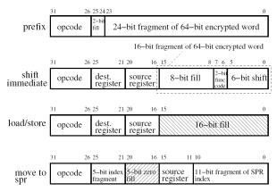
Notes: An extra 'prefix' instruction has been added to contain the bits of an encrypted immediate that do not fit in a following instruction, and the shift immediate instruction has been respecified to allow it to contain 16 bits of an encrypted shift that also incorporates the subfunction specifier. The displacement field in a load/store instruction is ignored, as is the designator register field in a move to/from SPR instruction.
