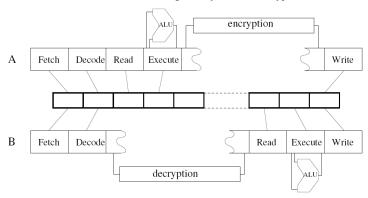
Figure 5 Pipeline integration, showing shadow units for user mode
