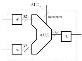
Note: Decryption units  $(\mathcal{D})$  are shown on inputs and encryption unit  $(\mathcal{E})$  on the output of an unmodified ALU.
