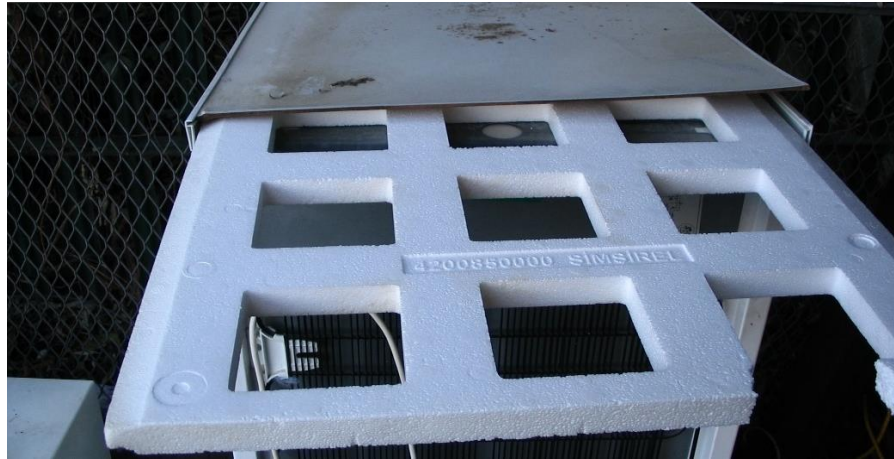
Figure 3.1 Polystyrene panel used in refrigerator construction.
