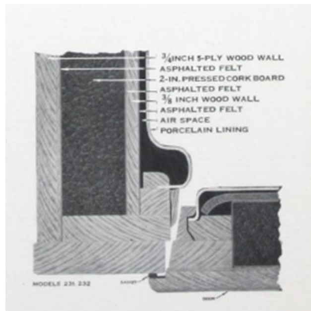
Figure 2.4 Cross-section illustrating the insulation materials used for the side-wall and door in a 1920's Kelvinator refrigerator (Kelvinator Corporation, 1926)
