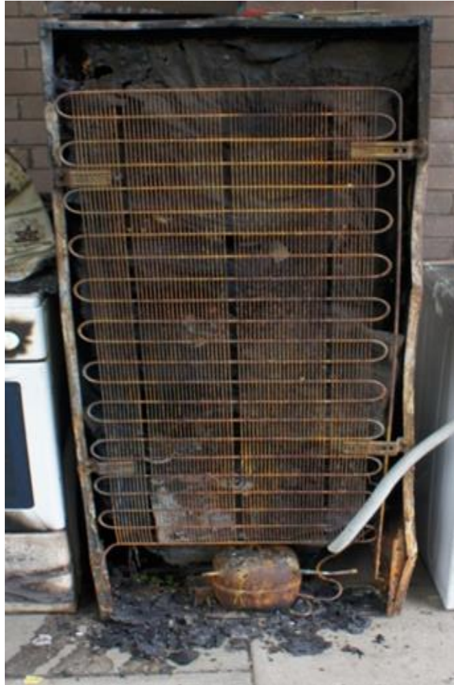
Figure 5.18 An example of a fire damaged appliance which was recorded as a defrost switch failure, illustrating the severity of the damage caused. (LFB Fire incident no 137039131 10/2013)
