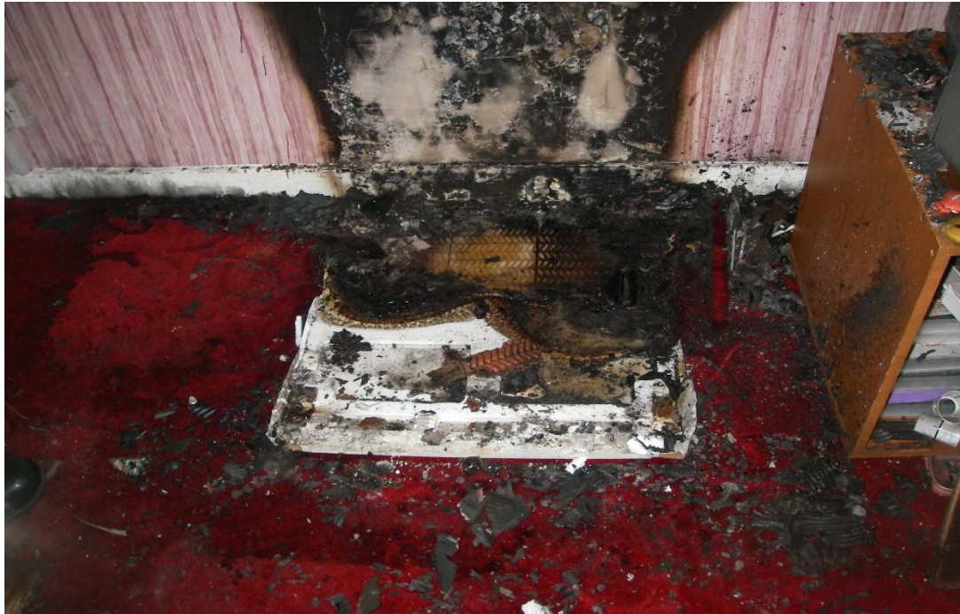
Figure 3.12. With the refrigerator removed, the remains of a base polystyrene and cardboard packing tray is observed. Packing materials are commonly found left in situ by owners', often years after installation.
