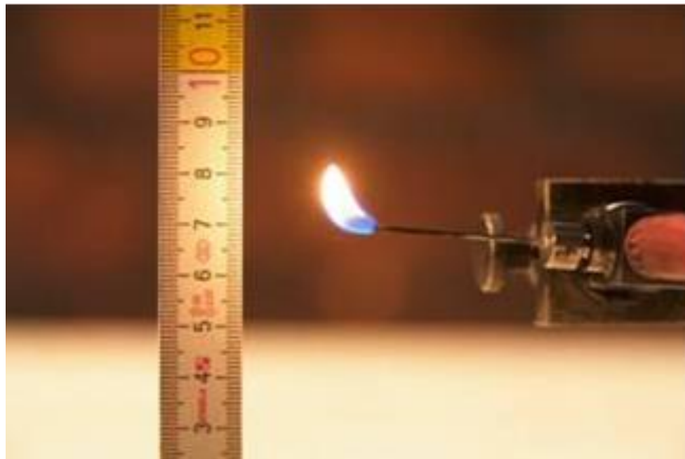
Figure 2.10 The IEC TS 62441 needle flame test Beard and Goebelbecker (2007)
