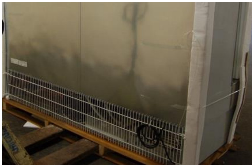
Figure 7.4 Grill guard across compressor housing.
