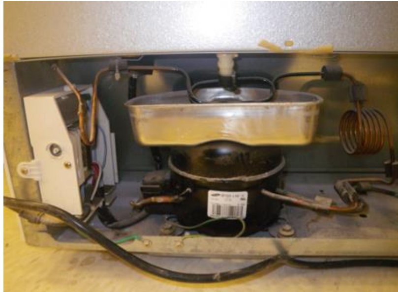
Figure 7.5 Example of a metal evaporation tray positioned above the compressor.
