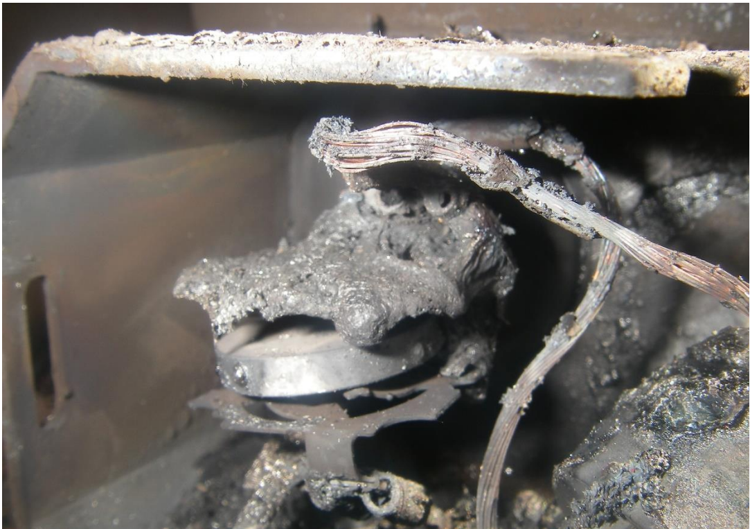
Figure 3.17. Close up of compressor positive temperature coefficient (ptc) switch showing side wall of pill
