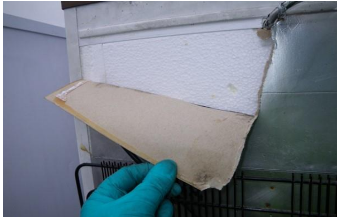
Figure 6.7 An example of metallised cardboard covering the rear wall foam insulation of an appliance.
