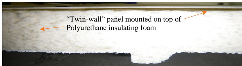
Fig 6.11 Twin-wall panel mounted on insulating foam viewed sideways.
