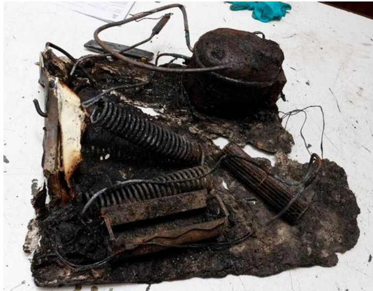
Figure 5.27 The remains from an integrated appliance fire. (LFB Fire incident no 133116151 2015)
