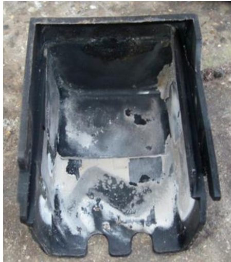
Figure 5.7 Build-up of adipic acid inside the cover of a PTC switch.
