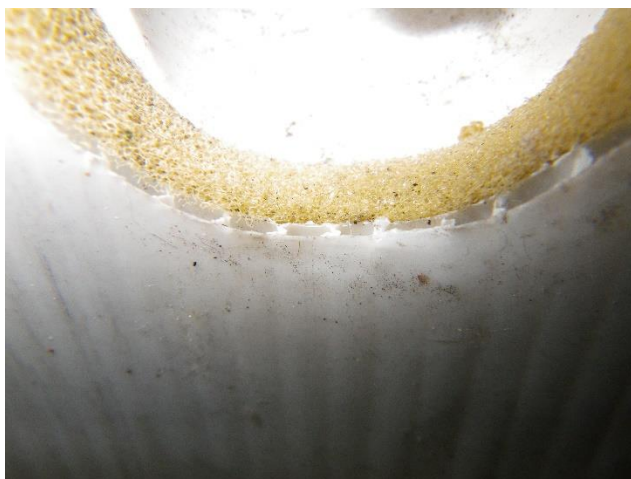
Figure 6.9 The twin-wall back panel cut to provide an outlet for water to drain through the rear wall of the appliance. The appearance is similar to joined plastic straws.
