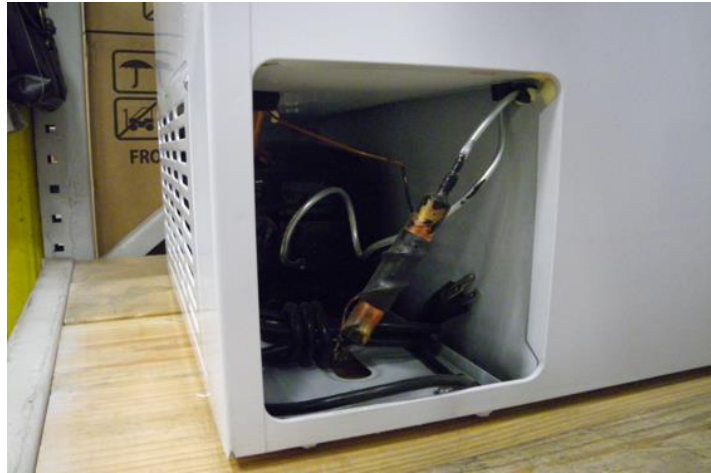
Figure 7.6 Example of using interior metal compartmentation to prevent fire spread from any potential component failure reaching the insulating material.
