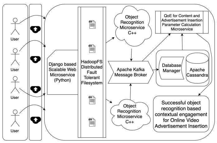
Figure 2. Overall Architecture for SuperEye Object Recognition based Contextual Engagement Online Advertisement Insertion System
