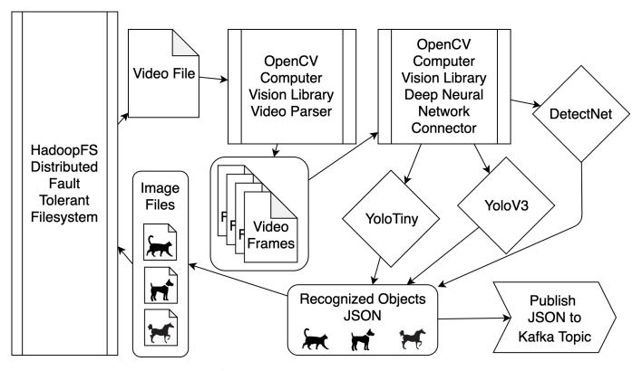
Figure 1. Architecture and Algorithm I for SuperEye Core Functionality, Object Detection and Recognition Microservice
