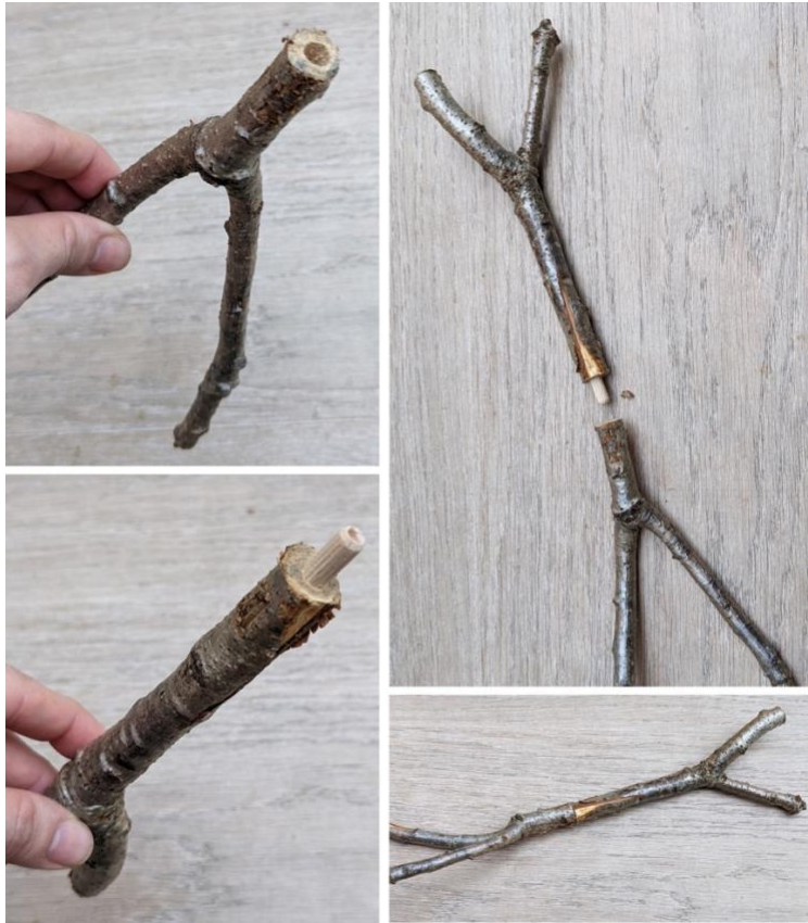
Figure 16: Wooden dowel joint experiment on two thin tree forks.
