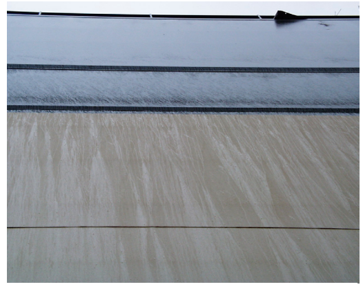
Fig.2 Horizontal steps, typically up to 40 mm high, in the external surface of the hull
