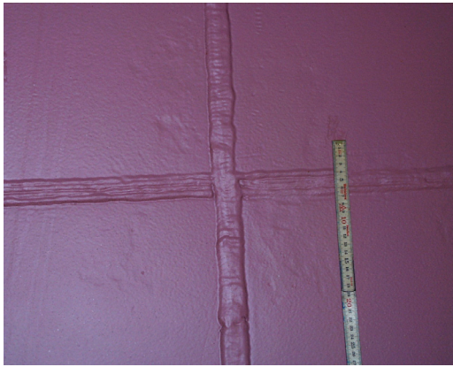
Fig.1 Welds on the exterior surface of a hull, 20 mm wide and up to 10 mm proud of the surface
