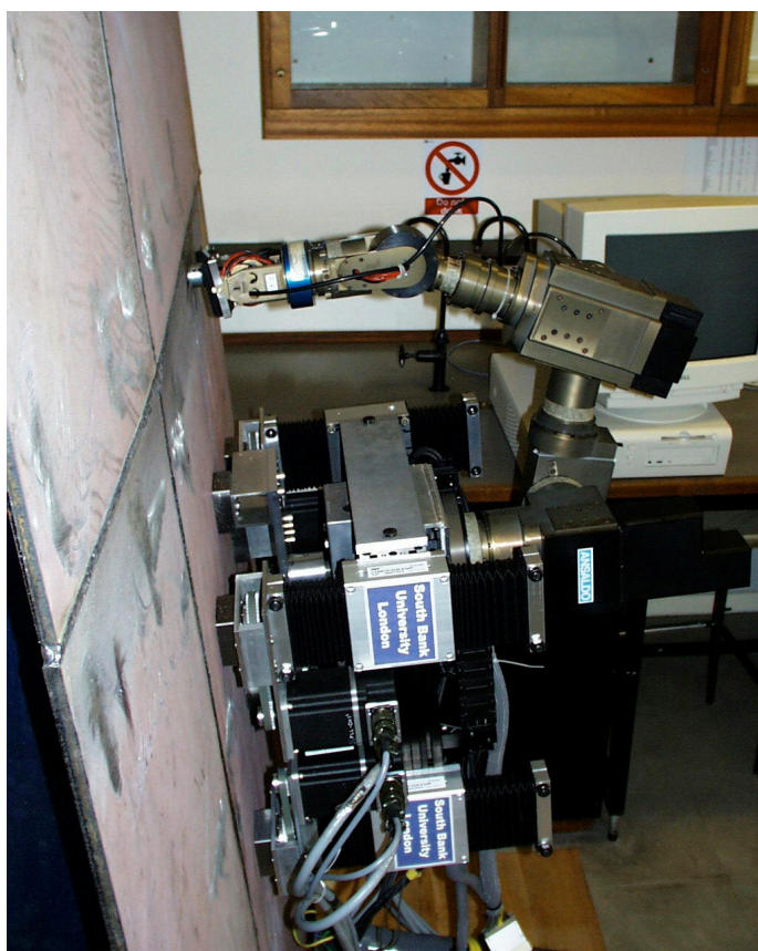
Fig.4 Climbing Robot Carrying the ANSALDO 7 DOF Arm on a Hull Mock Up
