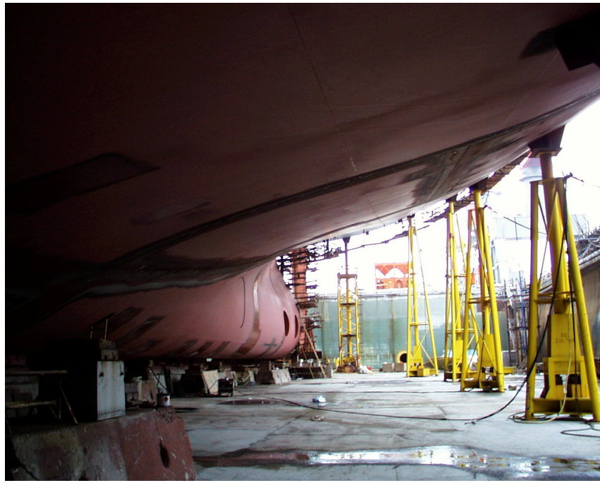
Fig.3 Stern section of a hull, showing the smallest curvature to which the robot must adapt
