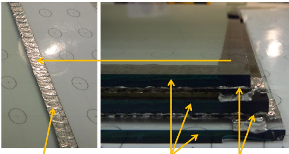
Primary edge seal with an approximate height of 1 mm
