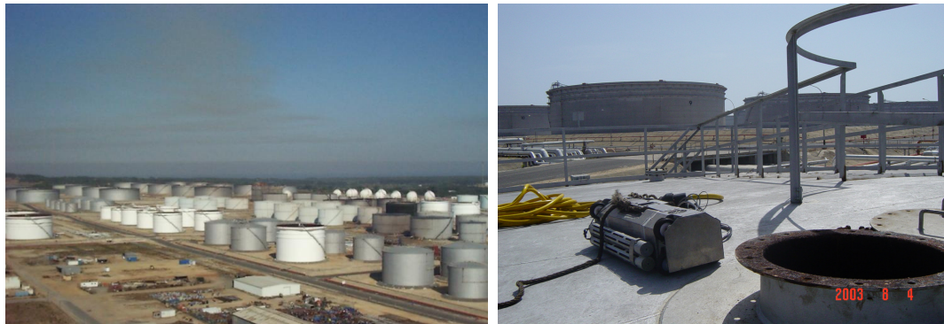
Figure 4: A tank Farm and the ROBTANK robot on a storage tank roof next to entry hole
