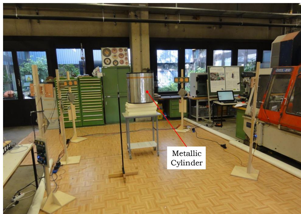
FIGURE C.13: Picture of the machine hall localization measurement with an additional scatterer
