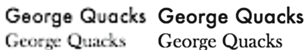
Fig. 5 Enlarged nine-point Futura and Baskerville fonts on an 86-PPI screen ( left ) vs the same on an iPad3 with 264 PPI ( right ). With more than nine times resolution, the fine details of text are legible
