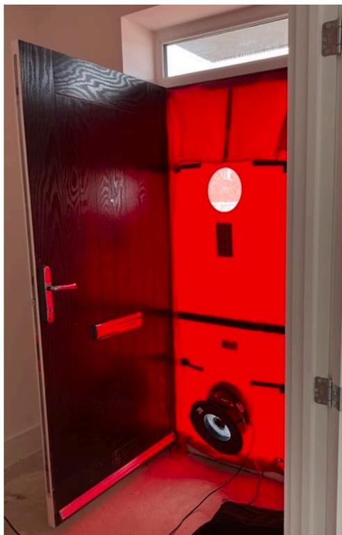
Fig. 3. Fan Pressurisation set-up.
