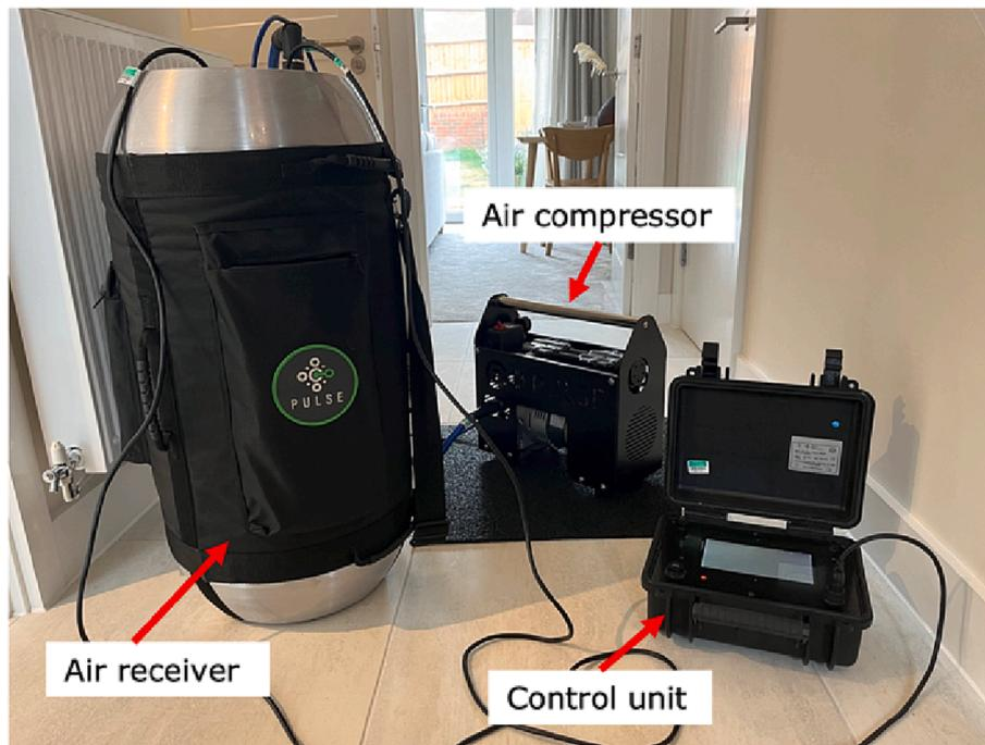
Fig. 2. Pulse set-up.
