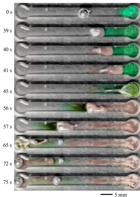
46 180 Figure 6. Snapshots of the motion of a Galinstan drop in 1 mol/L HCl solution with the addition of \text{CuCl}_2 .
