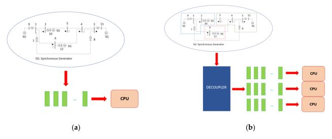
**Figure 1.** Exemplification of sequential and parallel computing: (a) the power system equations may be solved only sequentially; (b) the power system equations are divided into blocks and solved separately (e.g., the equation related to the inertial and primary response of the generators to a system frequency variation are decoupled and may be solved in parallel separately).
