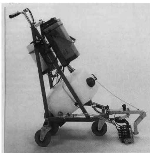
Fig 2. Manual plate tester used for testing plates at present
