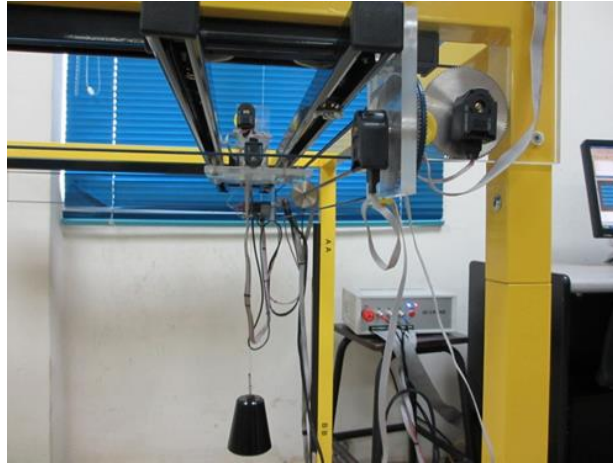
Figure 1. The laboratory 3D gantry crane
