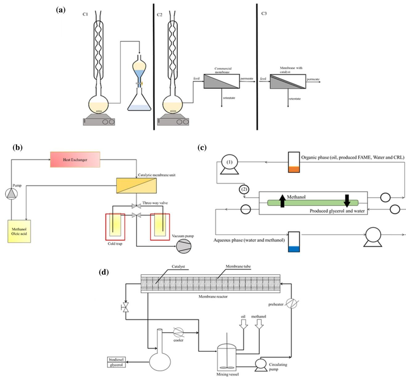
**Fig. 1** (a) Configurations for the transesterification reaction: (C1) conventional reaction using the heterogeneous catalysts dispersed in the bulk solution followed by separate standard phases partition; (C2) reaction with the heterogeneous catalysts spread in the bulk solution coupled with in situ continuous filtration performed with a com-
