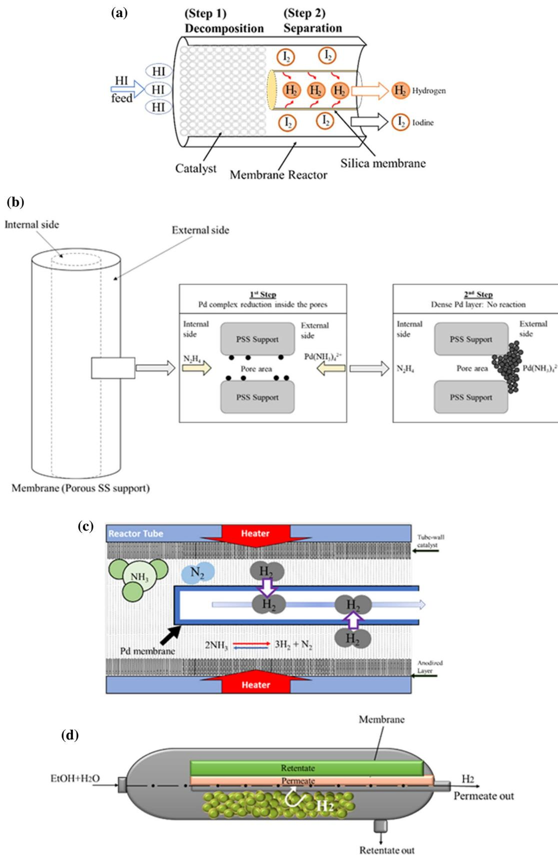
**Fig. 2** (a) Membrane reactor for hydrogen iodide decomposition; (b) pore plating technique; (c) tube-wall catalytic membrane reactor; (d) catalytic membrane reactor
