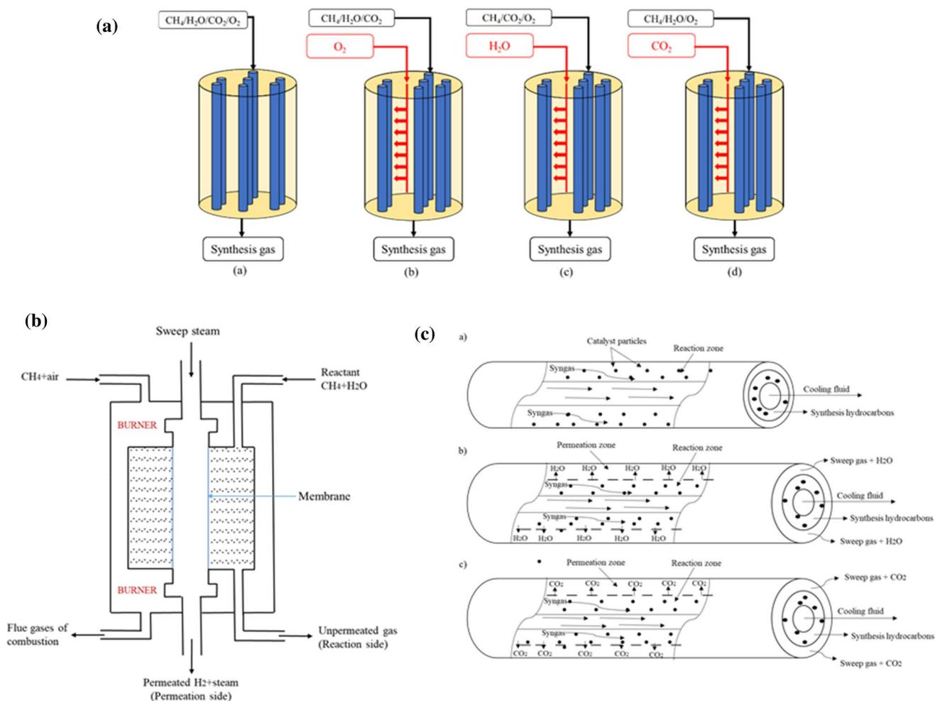
**Fig. 3** (a) a. Methane tri-reformer, b. microporous membrane reactors with  $\text{O}_2$ , c. microporous membrane reactors with  $\text{H}_2\text{O}$  and d. microporous membrane reactors with  $\text{CO}_2$ ; (b) membrane reactor;
