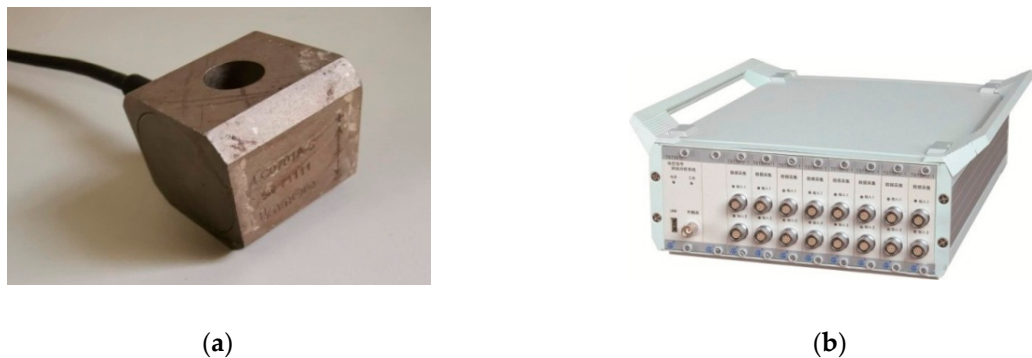
Figure 28. (a) Accelerometer; (b) Data acquisition device.
