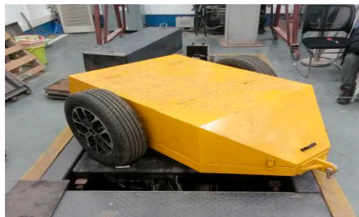
Figure 31. The single-axle test vehicle is tested on a shaking table.
