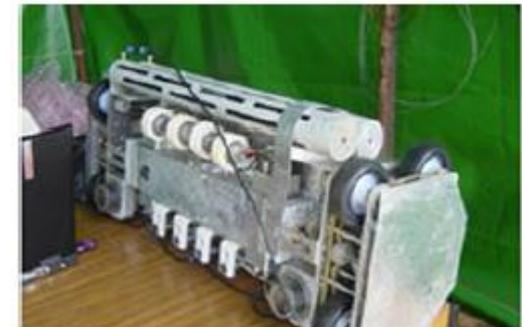
**ROBTANK: Mobile in-service robot enters through manholes on the floating or fixed roof of a storage tank to inspect its floor and walls**
