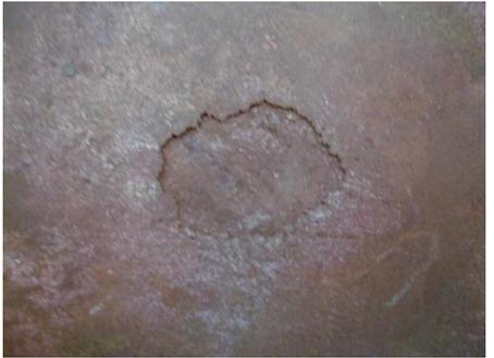
Manual tank floor inspection, underside corrosion defects
