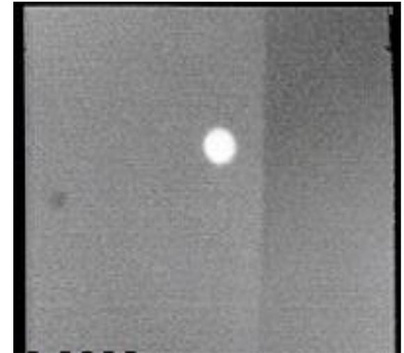
Thermographic detection of loose rivets
