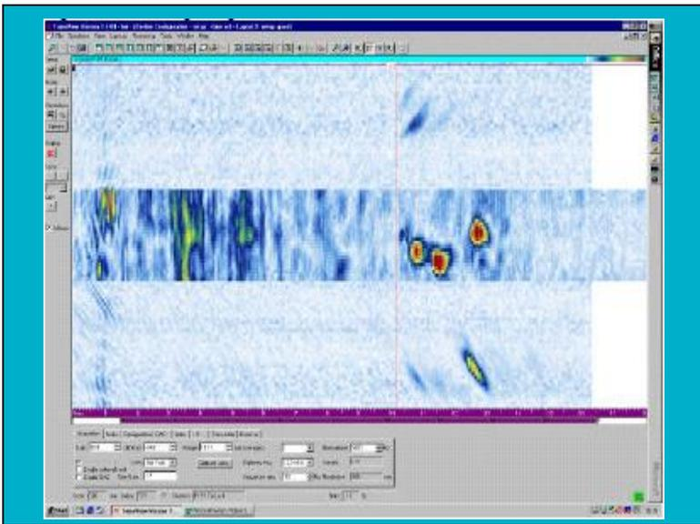
ULTRASONIC PHASED ARRAYS to inspect rivets on aircraft, ROBAIR project
