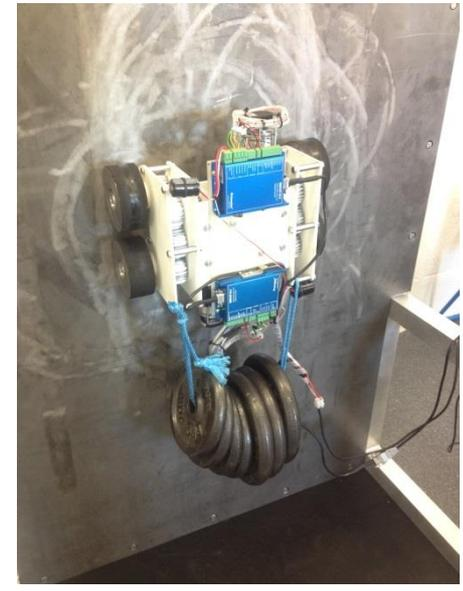
**LHS: Advanced wireless wall climbing robot for the inspection of welds on ship hulls. RHS: Magnetic Adhesion Concrete Climber**
