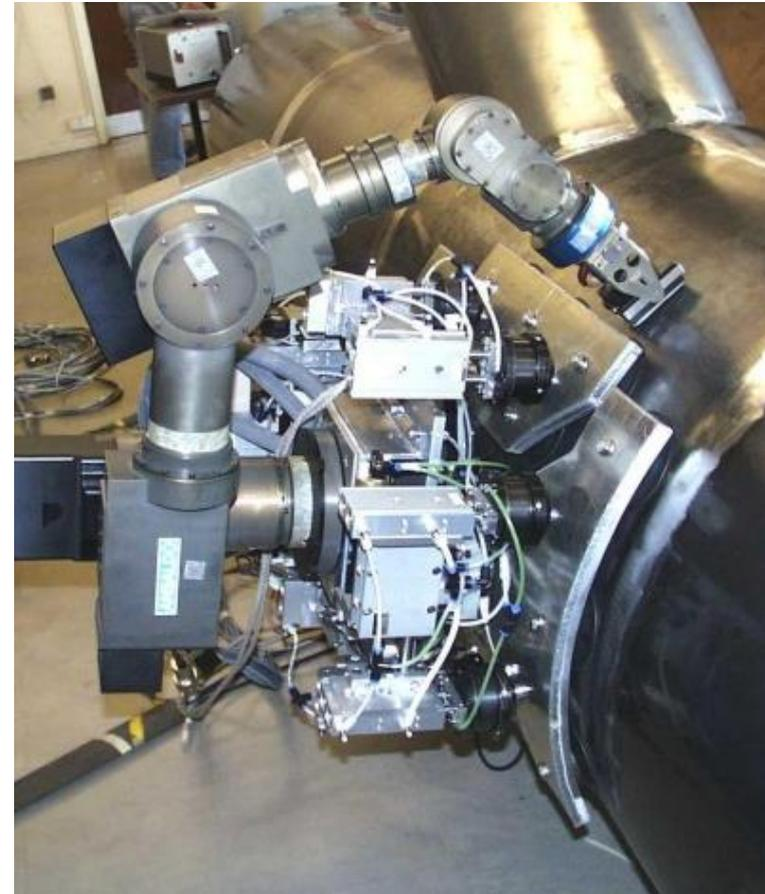
Some previous wall climbing robots for NDT developed by LSBIC
