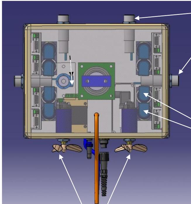
Ultrasonic range finders for detecting walls and strengthening plates
