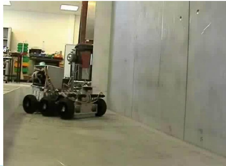
**FPSO swimming and floor inspection wheeled robot to inspect tank floors and welds on strengthening plates**
