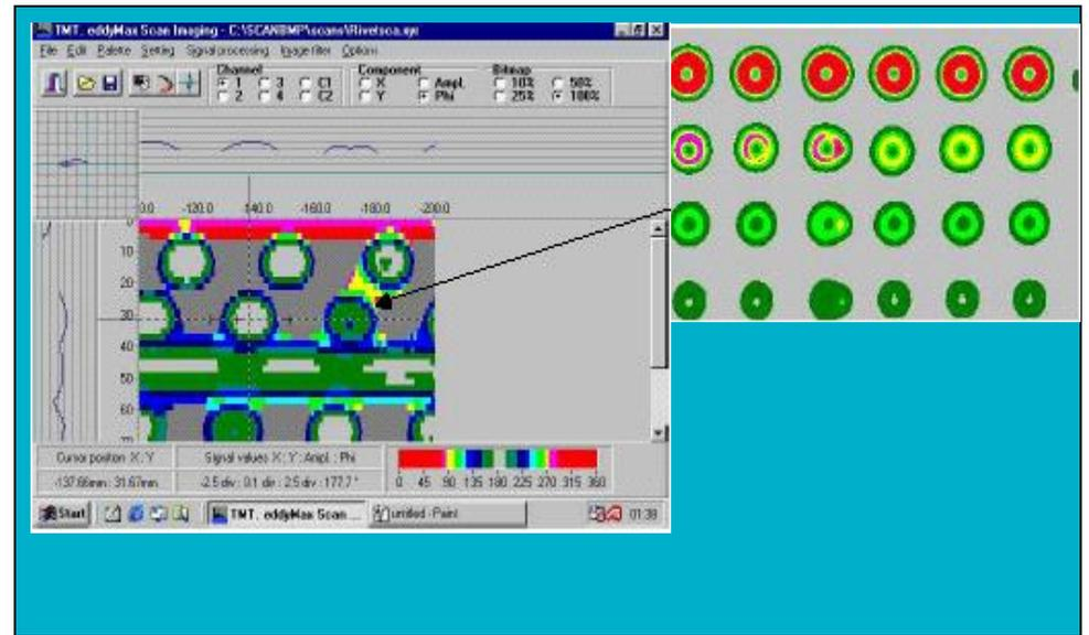
EDDY CURRENTS inspection of rows of rivets on the wings and fuselage of aircraft, ROBAIR project
