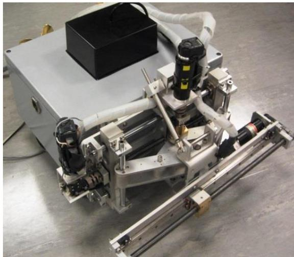
Wall climbing robots for NDT developed by LSBIC that use permanent magnets for adhesion
