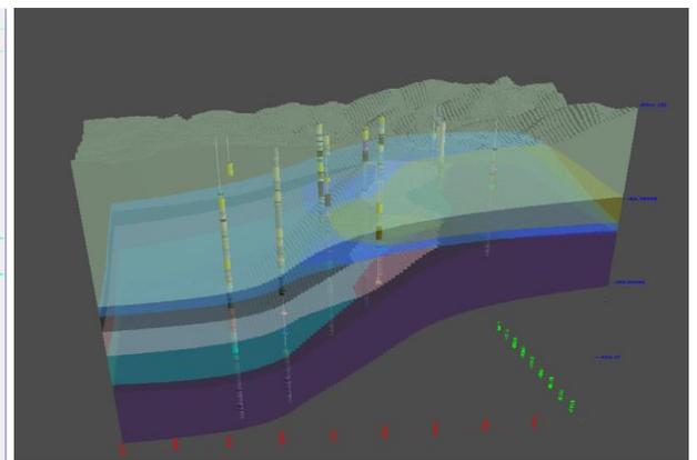
Figure 4: A simplified 3D model from correlating the borehole data. Colours represent subsurface formations.
