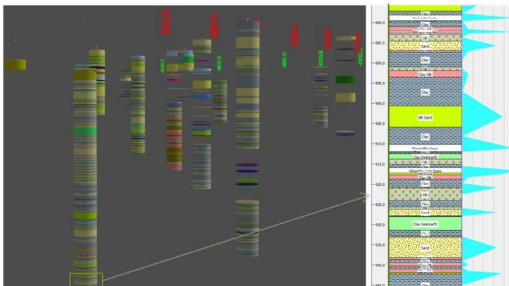
Figure 3: Digitised boreholes using Groundhog. Colours show different lithologies for a small section, lithology vs depth and a curve for transmissivity in light blue.
