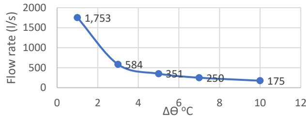
Figure 12: Required flow rate for storing 7MW of heat.
