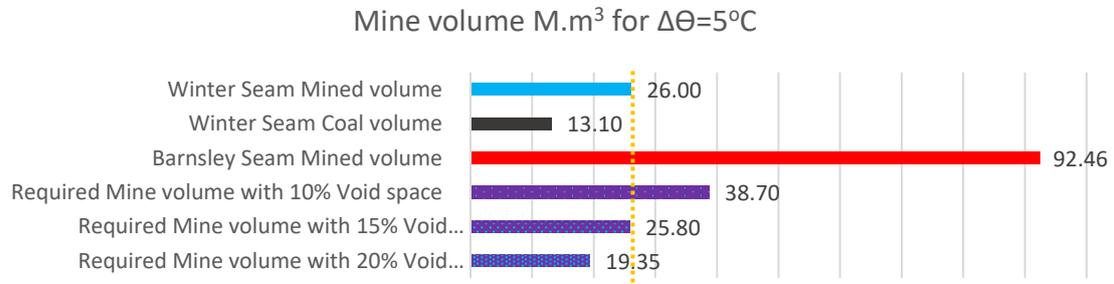
Figure 14: Available mine volume vs required mine volume to accommodate required amount of water for  $\Delta\theta=5^\circ\text{C}$ .
