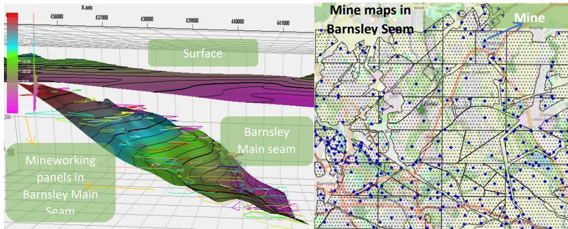
Figure 5: Mineworking panels in Barnsley main seam, right 2D, left, imported to 3D grid model and interpolated.
