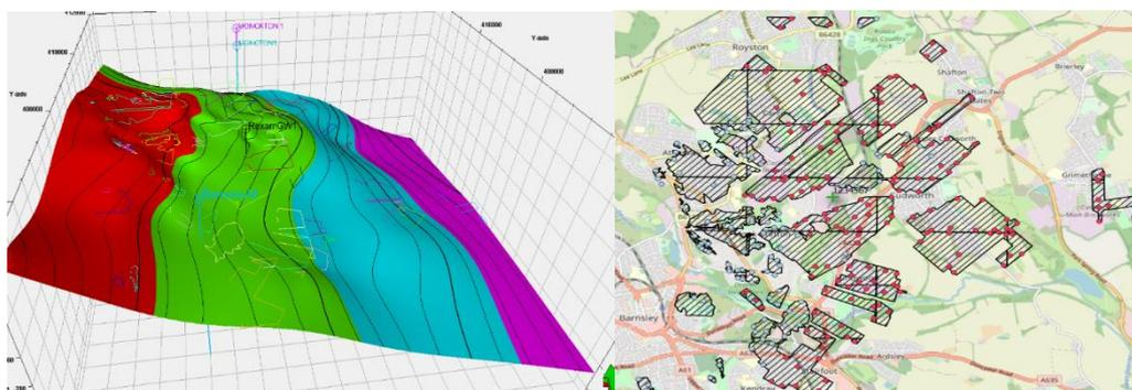
Figure 13: Mineworking map in Winter seam from the top (right-hand-side) and in 3D (left-hand-side)
