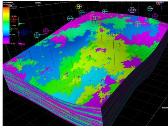
Figure 9: Permeability model, from top of the Winter Seam - cold source
