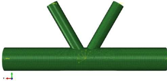
Figure 7.7 K-Type Tubular Joint Model: \beta = 0.5 , \gamma = 15 , \theta = 60^\circ
