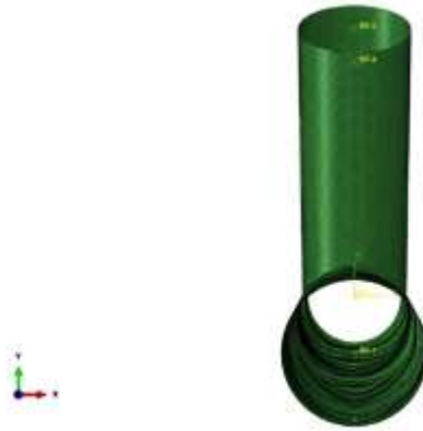
Figure 6.13 AMOCO K-Joint Finite Element Benchmark Model, X-Y plane view (generated in ABAQUS for Load Case 10)
