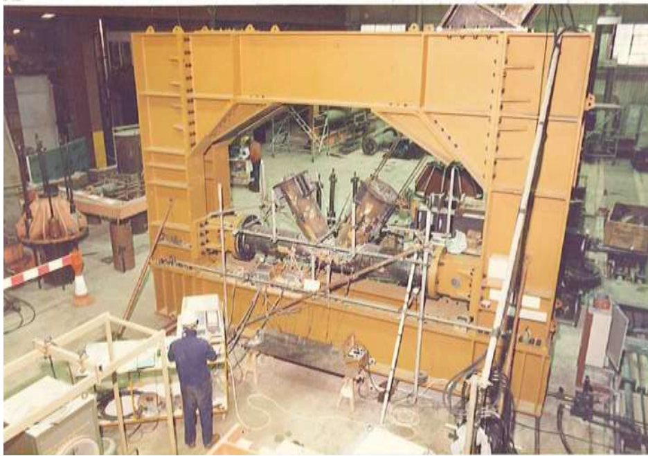
Figure 5.15 General Arrangement of Test Rig and Specimen (AMOCO K-Joint Tests 1983)
