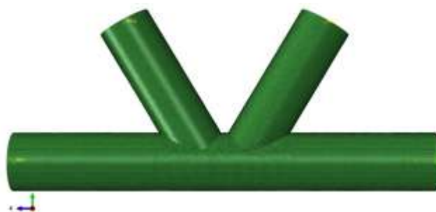
Figure 6.12 AMOCO K-Joint Finite Element Benchmark Model, Y-Z plane view (generated in ABAQUS for Load Case 10)
