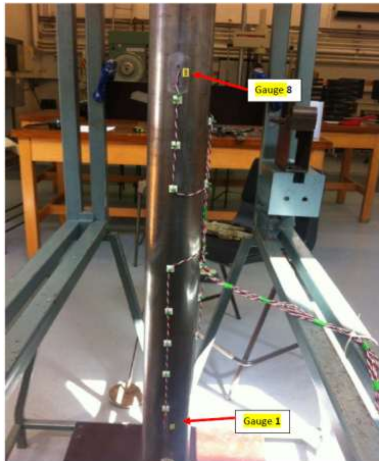
Figure 5.18 Transducer position (LSBU, 2015)
