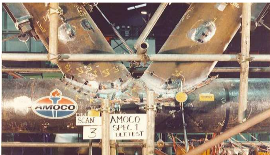
Figure 5.9 Specimen 1 under Ultimate Strength (Amoco K Joint Tests 1983)
