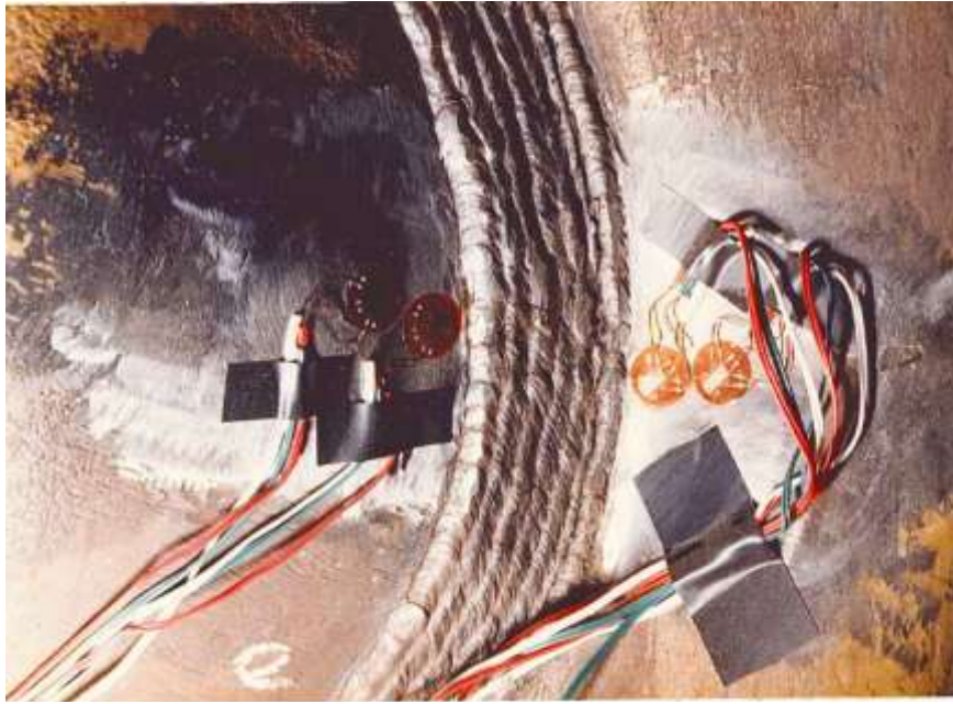
Figure 5.17 Details of Strain Gauges (AMOCO K-Joint Tests 1983)
