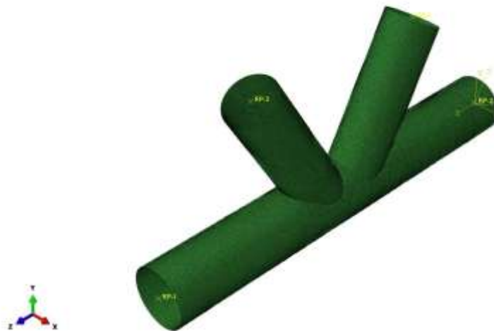
Figure 6.14 AMOCO K-Joint Finite Element Benchmark Model, X-Y-Z plane view (generated in ABAQUS for Load Case 10)
