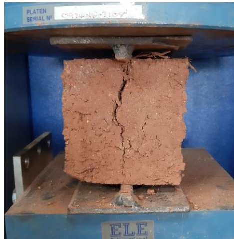
b. Tensile splitting strength test
