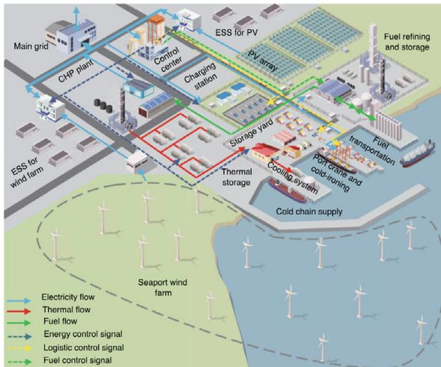
**FIGURE 1** A typical topology of future seaport microgrid [3].
