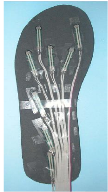
Figure 23: The placement of sensors and the developed foot sole.
