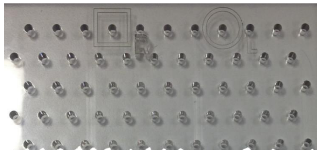
Figure 44: Top and left toe grooves on perforated sheet
