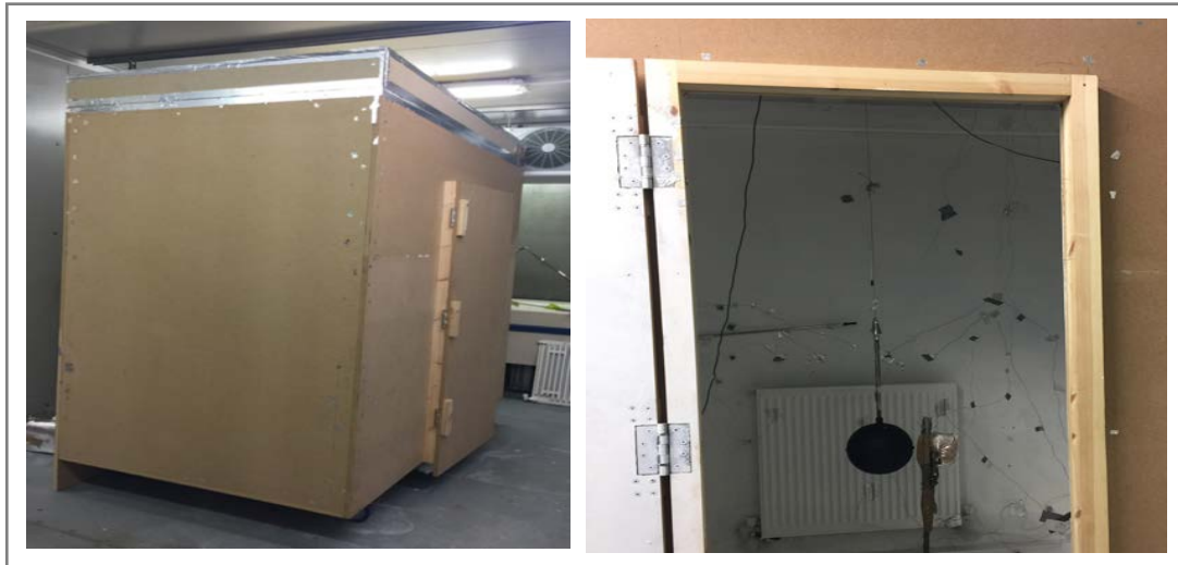
Figure 4.2: Booth with Tested Radiator
