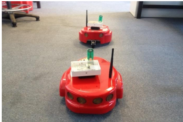
Figure 4: Two Amigo robots mounted with P410 in a testing environment.
