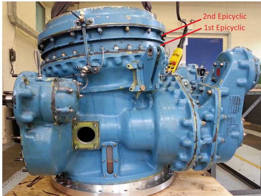
Figure 3.6: Demonstration of MGB epicyclic modules [109]
