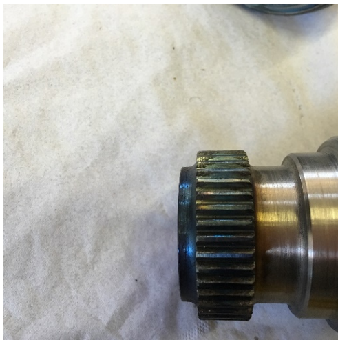
(a) Faulty shaft gear
