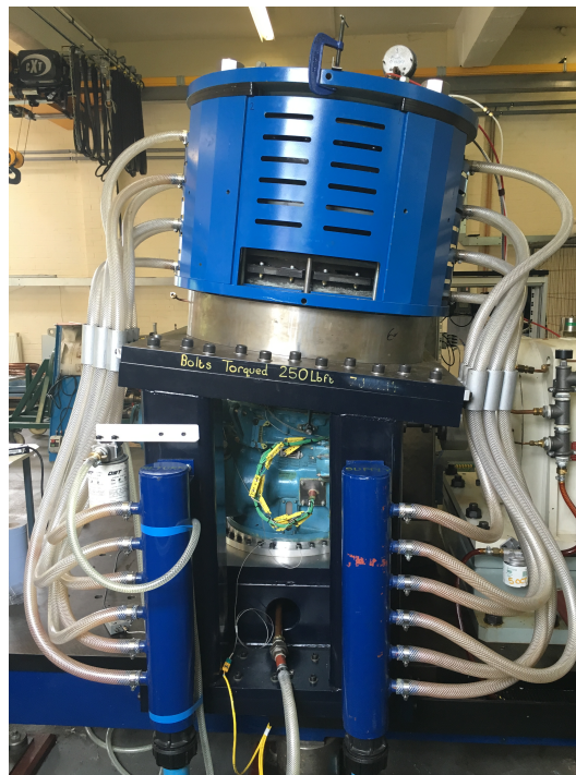
Figure 3.12: Dynamometer installed on top of MGB
