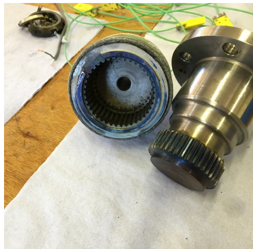
(b) Faulty shaft gear and ring gear
