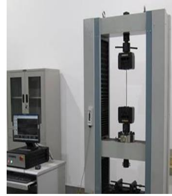
(a) Schematic diagram of tensile strength test (b) Electronic universal testing machine
