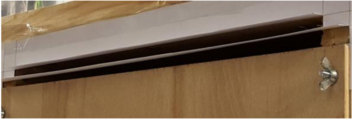
Figure 4.13 Developed test rig with paper louvres applied to the openings
