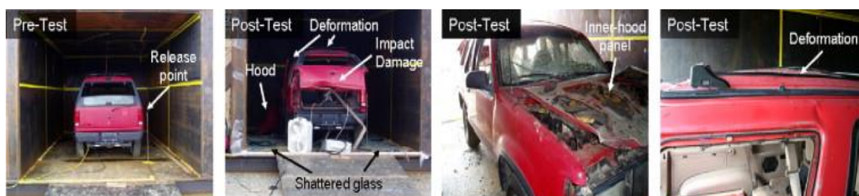
Figure 2.10 Pre-test and post-test photos of damage to the vehicle caused by an internal hydrogen–air deflagration (Merilo et al 2011).
