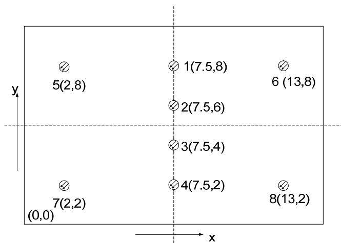
Figure 2. Positional coordinates (in cm) of eight thermocouples for temperature measurements on a steel substrate of dimensions 15 cm by 10 cm.
