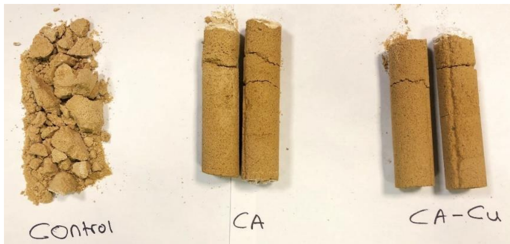
Figure 5 Typical image of a biocemented sand sample made from (a) Cementation Solution only as control, (b) Cementation solution and CA enzyme, (c) Cementation solution and CA-Cu nanoflower.
