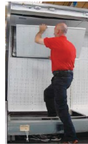
Cabinet is re-assembled with new and remanufactured parts
