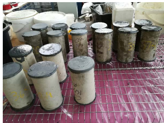
Fig. 3: Cylindrical concrete samples capped with sulphur.
