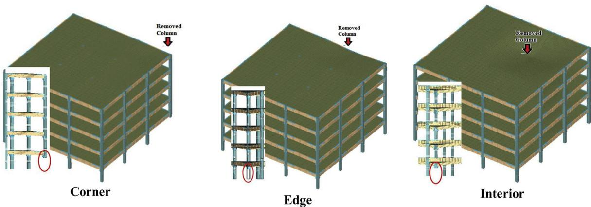
Fig. 13. 6 m and 9 m Spans Structures Overall Behavior After Removal of Corner Column in Ground Floor for all cases.
