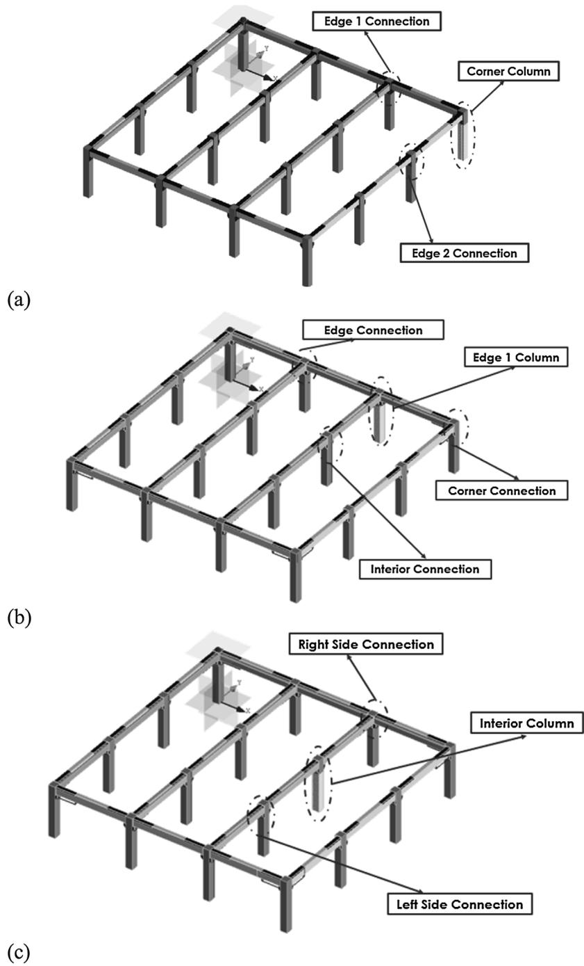
Fig. 9. Groun floor 3D model ELS model showing different column removal scenarios at : (a) corner, (b) edge and (c) interior.
