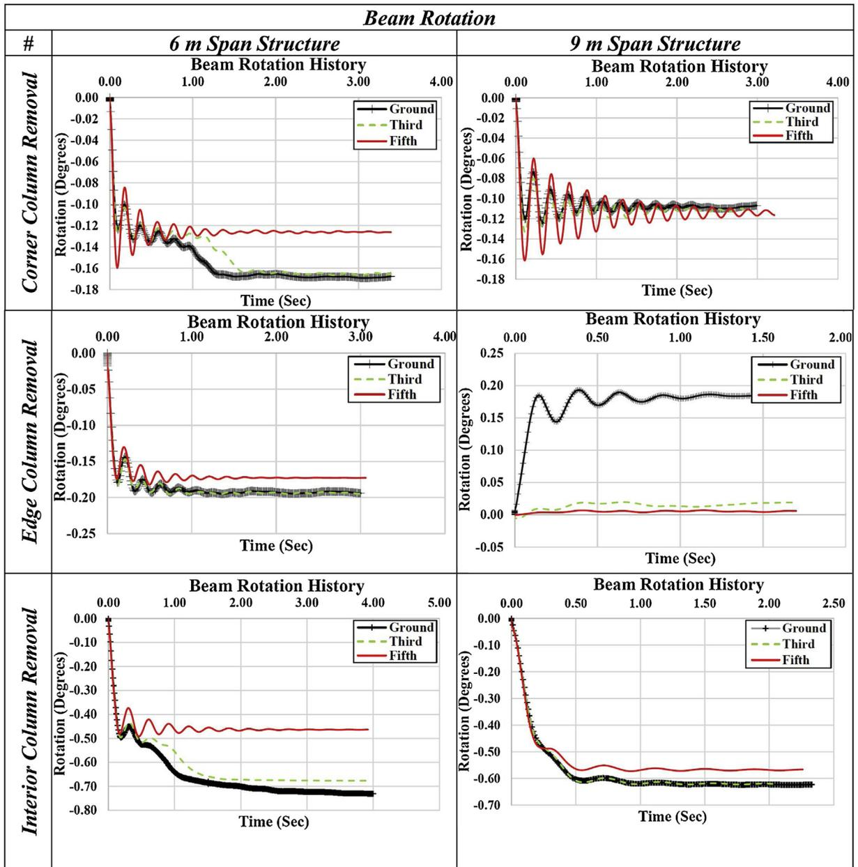
Fig. 18. Histories of Beam Rotation in Case of Corner, Edge, and Interior Columns Removal Scenarios for 6 m and 9 m spans structures for Ground, 3rd, 5th floors.
