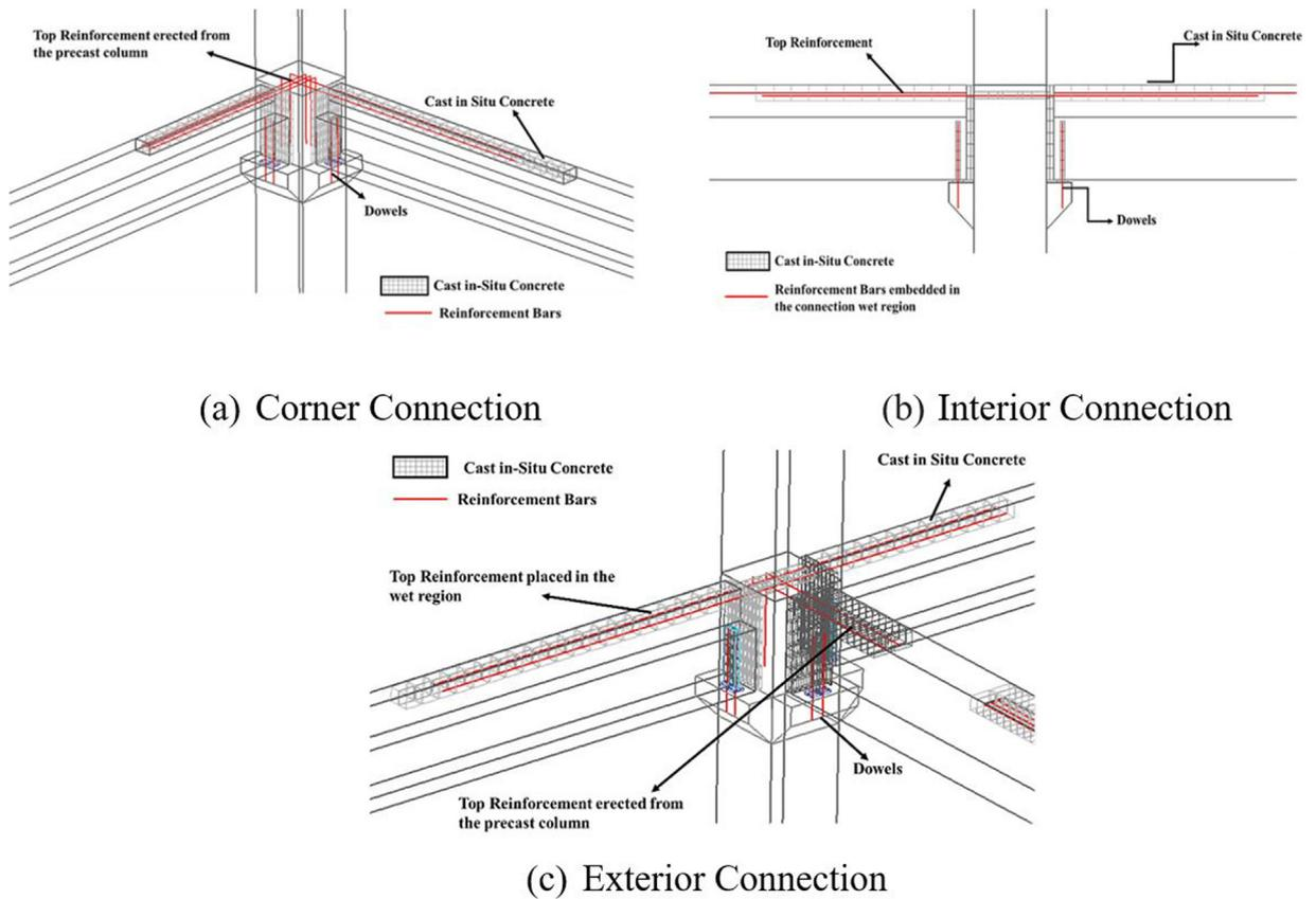
**Fig. 6.** ELS models for the studied connections (Corner, Interior, and Edge respectively).
