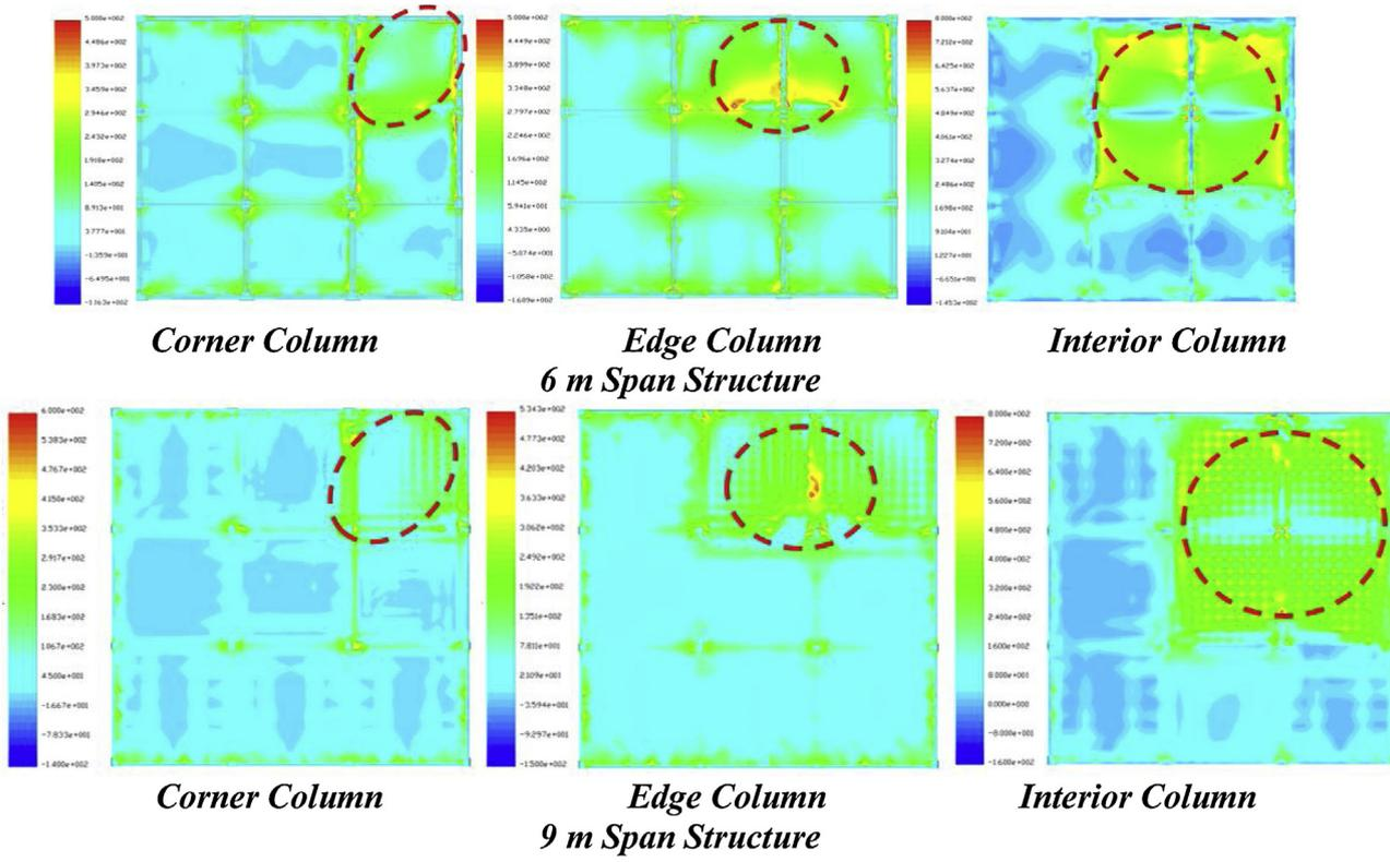
Fig. 15. Major principal stress contours in the slabs after column removal for ground floor for different column removal scenarios.
