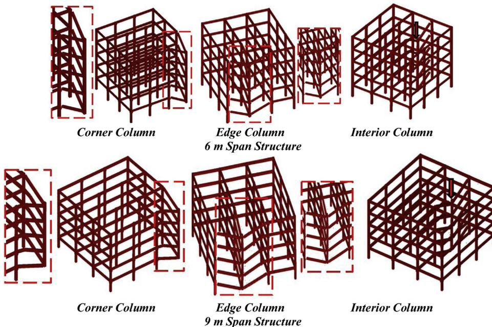
Fig. 12. Collapse after the support removal (3D bare frames).
