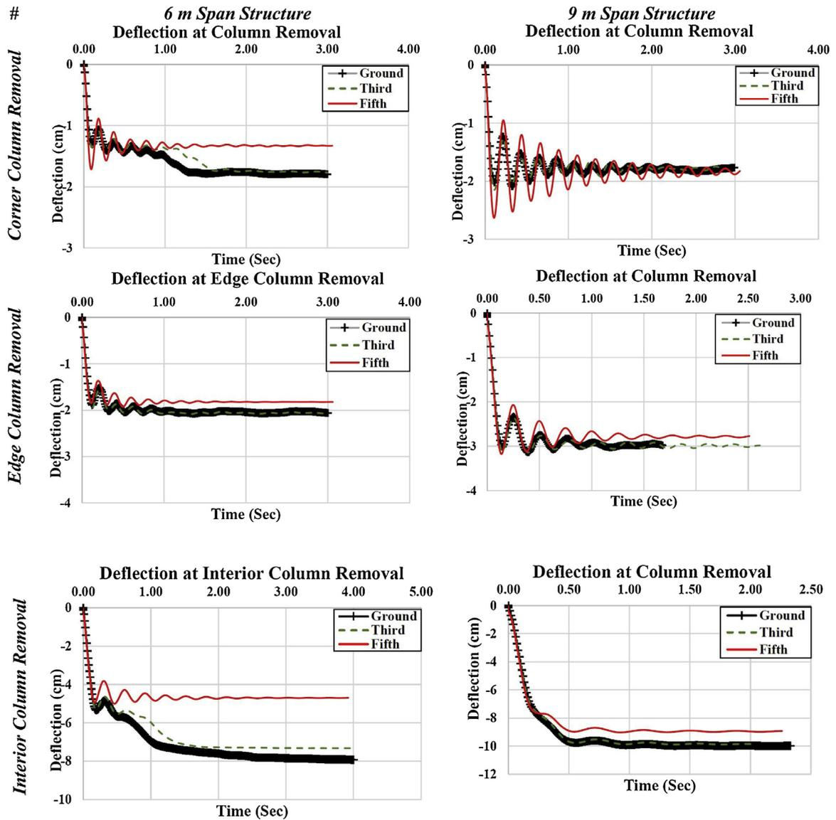
Fig. 14. Deflection at Column Removal for 6 m and 9 m Span Structures.
