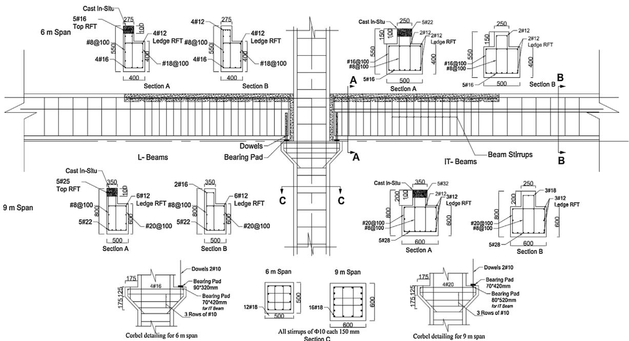
**Fig. 4.** Geometry and reinforcement details of the structure components.
