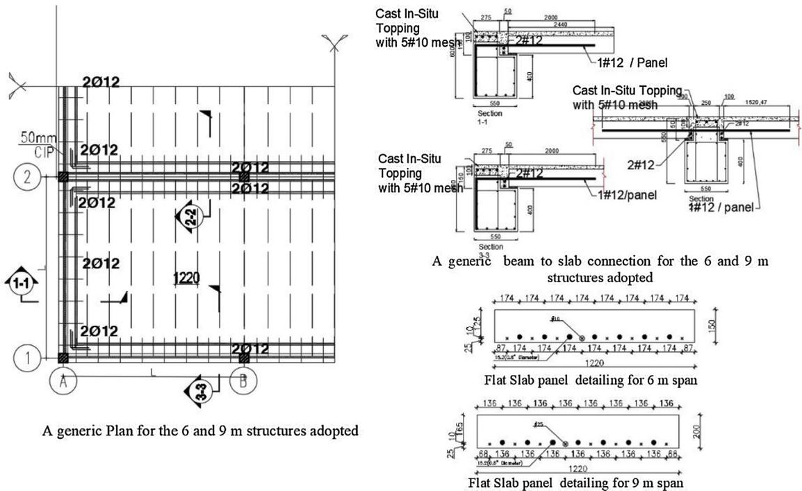
Fig. 5. Geometry and reinforcement details of the structure components.
