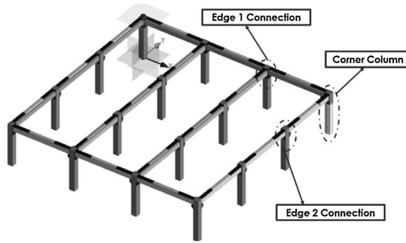
Fig. 7. 3D Model for the Removed Corner Column and the Adjacent Column.
