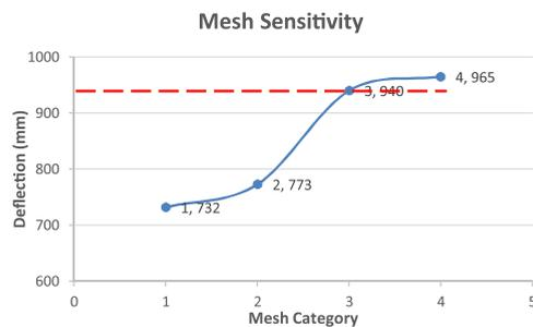
Fig. 8. Relation the Maximum Deflection Above the Removed Column and the Mesh Category.
