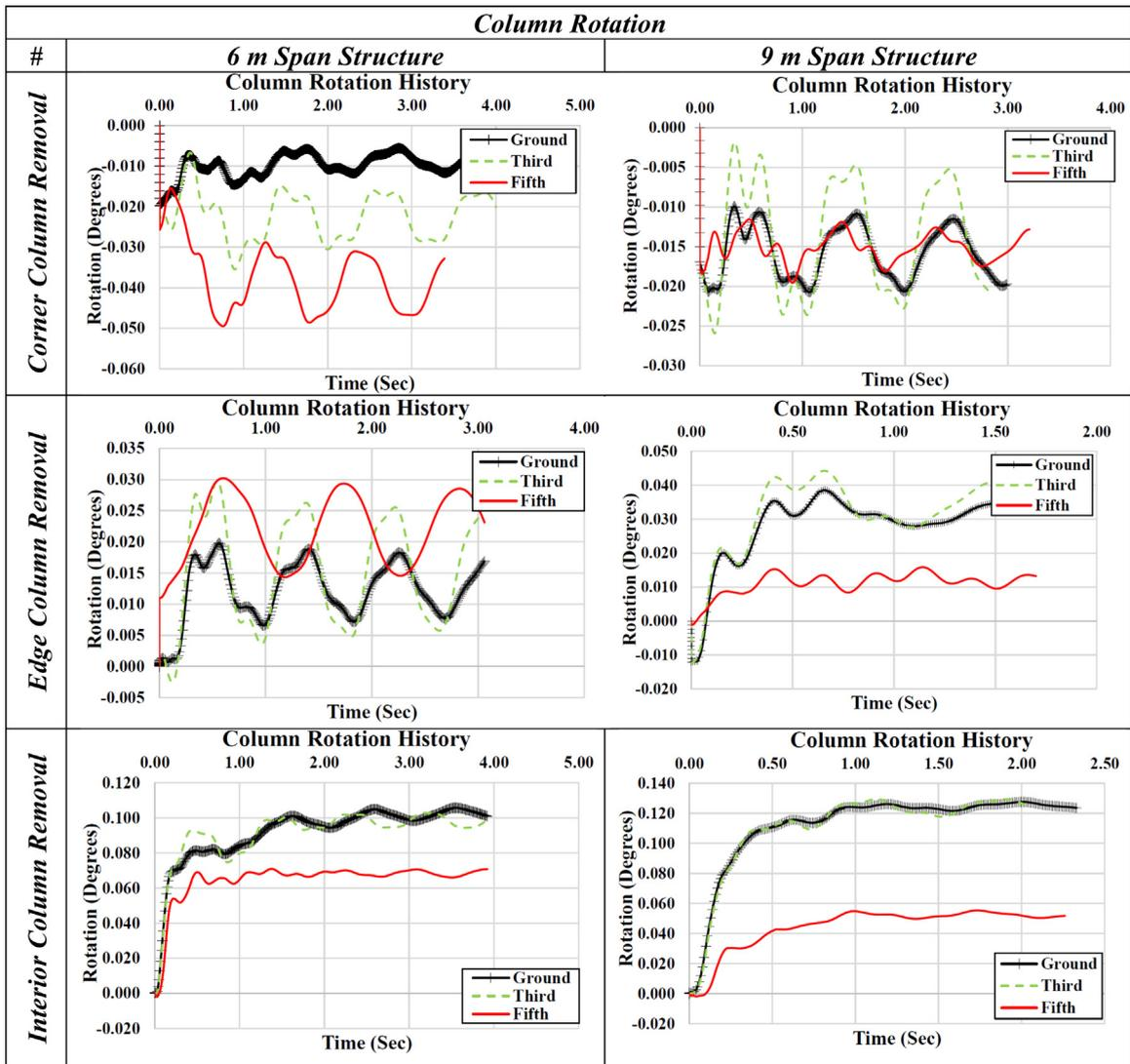
Fig. 17. Histories of Column Rotation in Case of Corner, Edge, and Interior Columns Removal Scenarios for 6 m and 9 m spans structures for Ground, 3rd, 5th floors.
