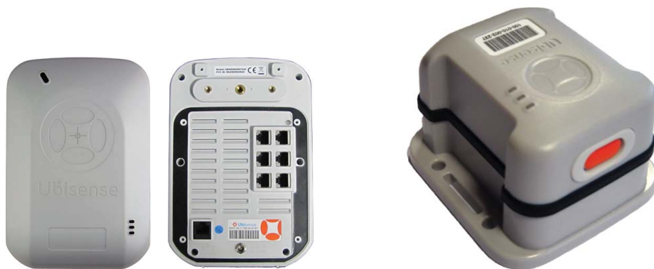
Figure 2.8: Ubisense sensor(left) and tag (right) [92]
