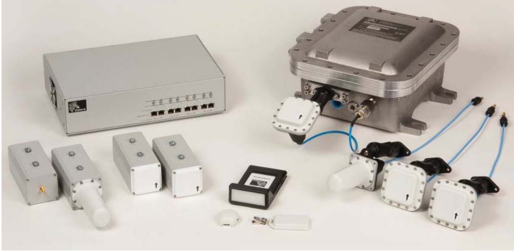
Figure 2.9: The Zebra DART UWB system [89]
