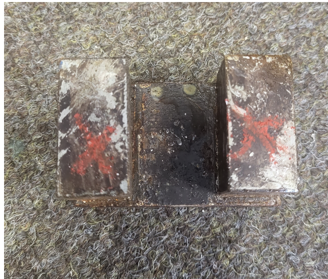
FIGURE 4.15: The opposite pole of the magnets marked to ensure that the direction of the magnets is correct.
