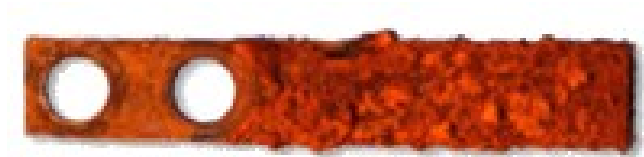
FIGURE 2.2: The corroded coupon that is reweighed to estimate corrosion damage.
