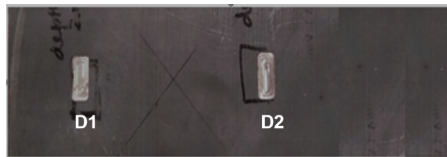
FIGURE 4.13: The mild steel plate with machined defects.
