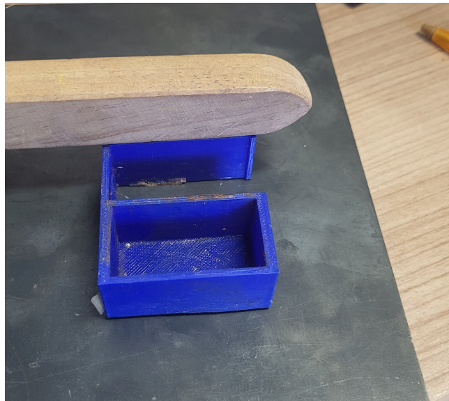
FIGURE 4.17: Wooden piece placed in the space between the magnets to avoid snapping.
